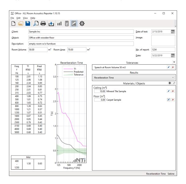
Designed for room acoustic experts, this comprehensive tool uses data gathered by the XL2 Sound Level Meter, and quickly returns graphical analysis of all measurement positions. Analyzing the measurement data and producing reports is straight-forward using the Room Acoustics Reporter software. Just drag & drop the XL2 measurement data into the software and print the report.
