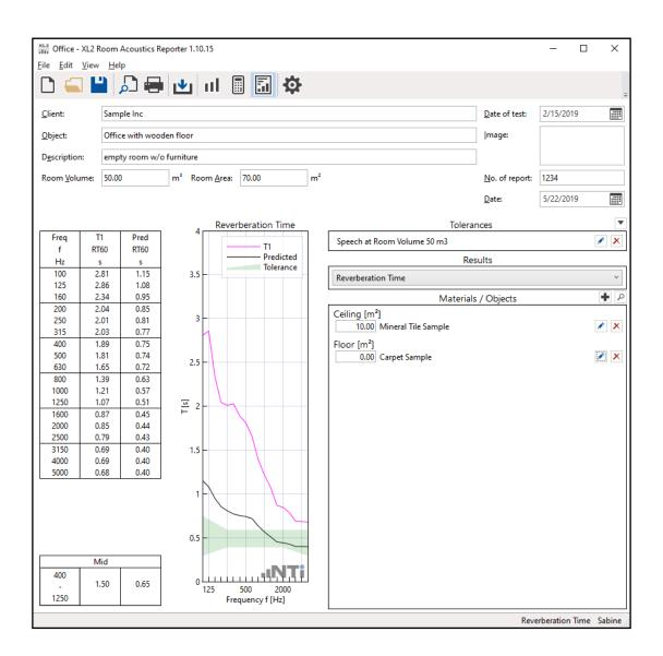
The result view displays the predicted reverberation time with the selected absorption material.
