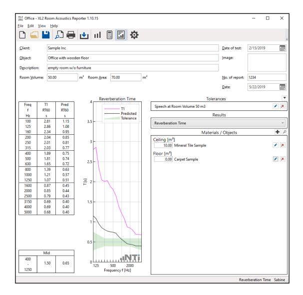
The result view displays the predicted reverberation time adding the entered absorption material.
