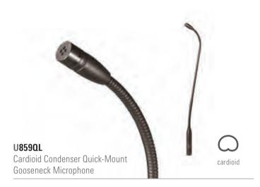
Designed to plug directly into a panel- or desk-mounted XLRF-type connector, the U8590L features an ultra-flexible small-diameter gooseneck and accepts interchangeable elements, available in cardioid, hypercardioid, omnidirectional and UniLine polar patterns. Equipped with self-contained electronics, the phantom-powered microphone also offers an 80Hz low-cut UniSteep® filter that reduces pickup of low-frequency ambient noise. The microphone is is 480.0mm long.
